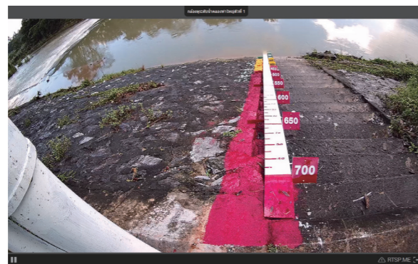
Figure 3: example picture from the city's CCTV camera with the indicator of water level in the city canal
